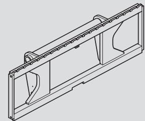
**TABLIER NORMALISÉ À DÉPLACEMENT LATÉRAL (SUR TABLIER INCLINABLE TI)**
